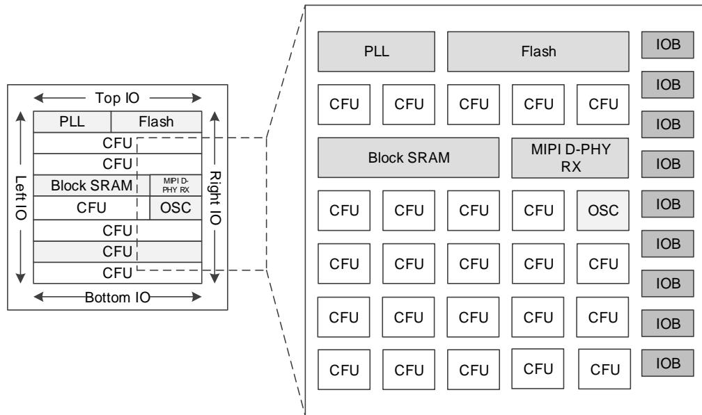
As shown in Figure 2-1 to Figure 2-3, the core of the FPGA is an array of logic cells surrounded by IO blocks. Besides, BSRAMs, DSP blocks, PLLs, an on-chip oscillator, and Flash resources that support instant-on are provided. As shown in Figure2-4, the GW1N-2 device is further embedded with a hard MIPI D-PHY RX core compared with other GW1N devices. See Table 1-1 for more information on the resources provided.
