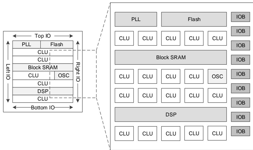
**Figure 2-3 Architecture Overview of GW1N-1**
