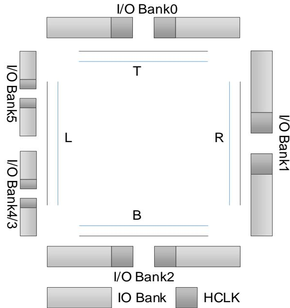
**Figure 2-23 GW1N-4 HCLK Distribution**
