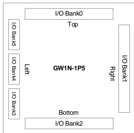
There are six banks in the GW1N-2 device, while in the case of GW1N-2 in the CS42, QN48H, MG132H, QN88, and CS42H packages,
