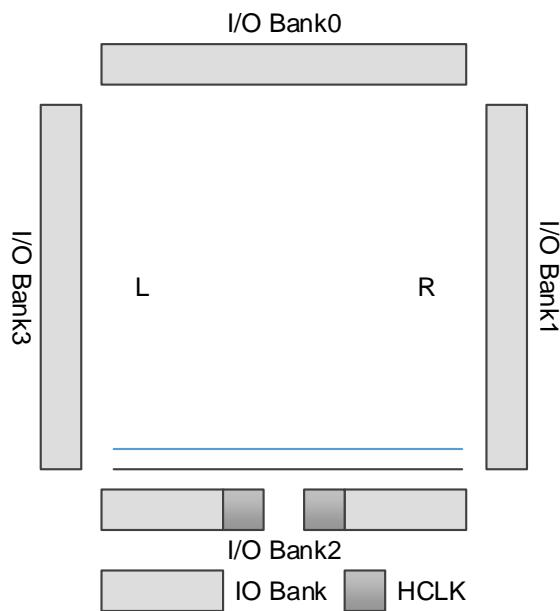
**Figure 2-22 GW1N-1P5/2 HCLK Distribution**
