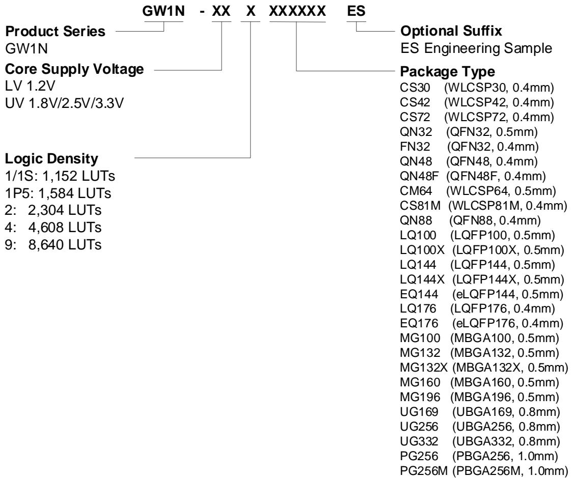
**Figure 4-2 Part Naming—Production**
