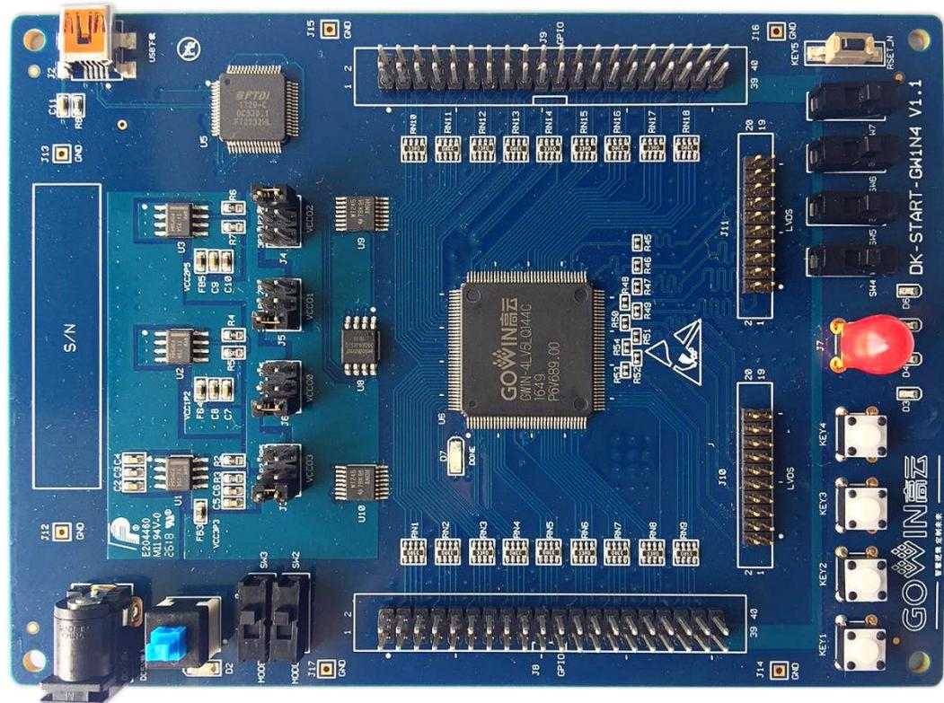
The Development board adopts the GW1N-LV1/2/4/6/9LQ144 devices of the GW1N series of FPGA products. It features a range of advanced features including low power consumption, instant start-up, high security, low-cost, and flexible extensions, all of which can effectively reduce the learning cost and help users quickly design and develop programmable logic devices.
